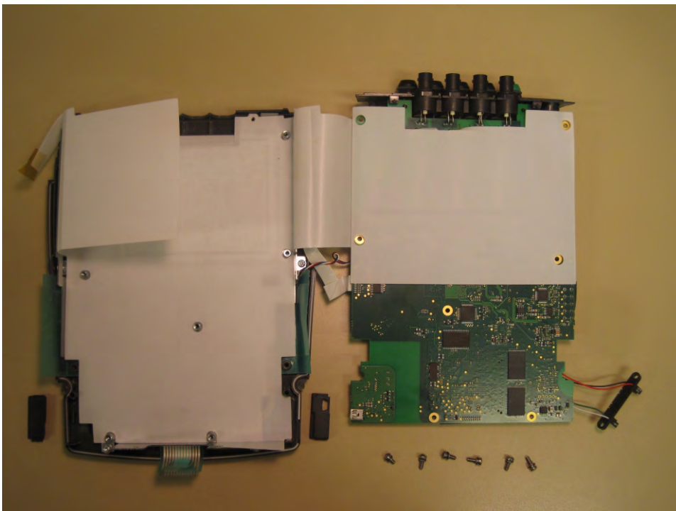
Fig. 6-3. Dismantling step 3 (PCA separated from chassis)
