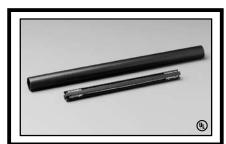
Simplify UF cable repairs after a trencher has damaged or destroyed a 7" to 10" section of UF cable. Utilize EPCO's Thick Wall Heat Shrink Tubing with sealant to make a quick and reliable repair. Eliminates epoxies, tapes or separate mastics and creates a waterproof, fully submersible splice. The kit includes one 4-position, 11.5" connector and one piece of heat shrink tubing, designed to splice and insulate 14 to 8 AWG UF cable.
