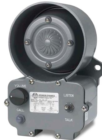
Designed for single-channel, two-way indoor and outdoor communication applications, Wall-Mount Intercoms feature integrated volume control, TALK/LISTEN switch, corrosion resistant cast aluminum housing with rugged powder coat finish (Type 4X, IP56 enclosure), reliable 25-watt speaker, and balanced line output. These heavy duty units are UL listed, CSA Certified and Marine rated; and available in 12 or 24VDC and 120 or 240 VAC, 50/60Hz models.
