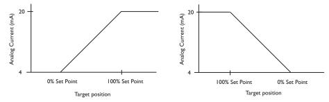
Note: If the distance between the 0% and 100% setpoints is less than 5% of the overall operating range, then the analog output will be automatically scaled to 5% of the operating range and the middle is placed between the 0% and 100% setpoints.
