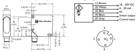
The control input (pin 5) can be used to disable the laser by connecting it to the +DC power supply (18...30V DC). The laser is shut down and both the discrete and analog outputs will retain their state. The control input (pin 5) can also be used to prevent setting changes to the sensor (lock out the Teach-in buttons) by connecting it to 0V DC. The sensor can be operated in the free-run mode by not connecting the control input (pin 5).
