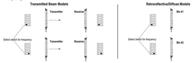
An additional method for dealing with sensor cross talk interference is by alternating the direction of transmitter/receiver pairs. The same effect can be achieved with the retro/diffuse model by setting the units up back to back.
