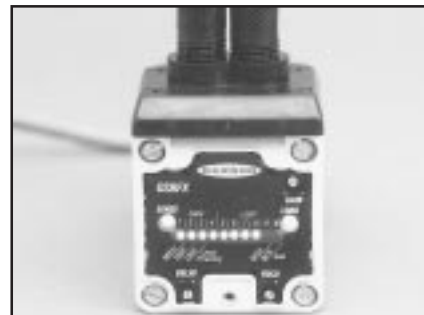
LIGHT condition example: D.A.T.A. system LEDs #1 through #8 lit.
