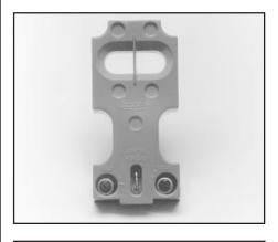
The logic module interconnects the power block and scanner block both electrically and mechanically using a unique blade-and-socket connector concept. It also provides the LIGHT/DARK operate function (except in the LM1) and the timing functions, all of which are fully adjustable.
