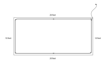
Consider using shorter length kits to build longer custom lengths. If one section should fail, a kit can be replaced (which maintains UL Listing) versus repairing a section, which voids UL.
