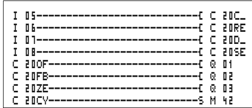
Figure 100: EZD circuit diagram with counter relay
