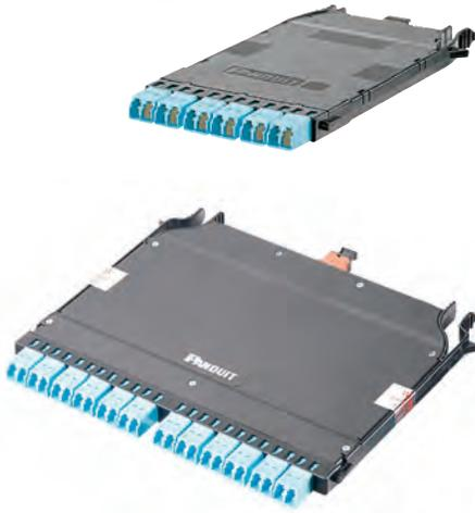
**Cassettes and FAPs** – Modular cassettes in either 6-port or extra wide 12-port configurations are part of the system, and FAPs for deploying a fiber infrastructure as you migrate to higher network speeds.
