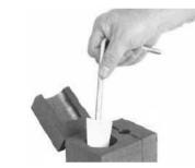
MOLD CLEANERS ARE USED TO CLEAN THE SLAG FROM MOLDS THAT ARE NOT SPLIT THROUGH THE CRUCIBLE.
