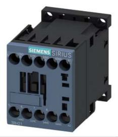
CONTACTOR RELAY, 3NO+1NC, AC 220V 50HZ, 240V 60HZ, SIZE S00, SCREW TERMINAL
