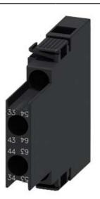
LATERAL AUX.SWITCH BLOCK,SIDE, 2NO, CURR.PATH: 1NO, 1NO, FOR MOTOR CONTACTORS, SZ S0 AND S2 SCREW TERMINAL R: 33/34, 43/44 L: 53/54, 63/64
