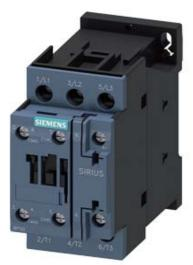
CONTACTOR, AC-3, 18.5KW/400V, 1NO+1NC, AC 110V 50HZ, 120V 60HZ 3-POLE, SZ S0 SCREW TERMINAL
