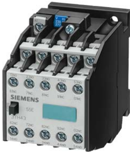
CONTACTOR RELAY 44E EN 50 011 4NO+4NC, SCREW TERMINALS AC OPERATION AC 120V 60HZ/AC 110V 50HZ
