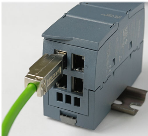
Figure 4-7 Inserting the IE FC RJ-45 Plug 180
