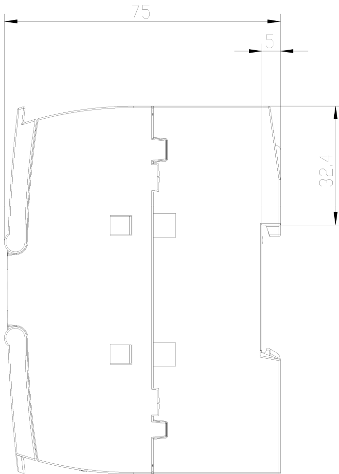
Figure 7-2 Dimension drawing, view from side
