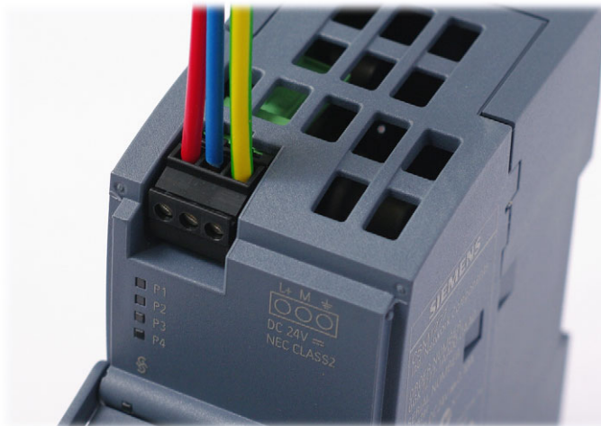
Figure 4-4 Connecting the power supply
