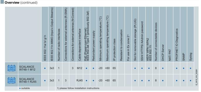
Function overview of the SCALANCE W client modules in accordance with IEEE 802.11n standard
