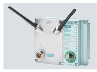
Interface module for handling communication between ET 200pro and host PROFINET IO controllers over Industrial Wireless LAN (IWLAN) radio networks for 2.4 GHz or 5 GHz with data transfer rates up to 54 Mbit/s.
