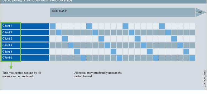
However, WLAN also provides a transmission mechanism based on standard WLAN in accordance with IEEE 802.11, which makes a defined data rate available to all stations. This means that access **by all stations** can be predicted.
