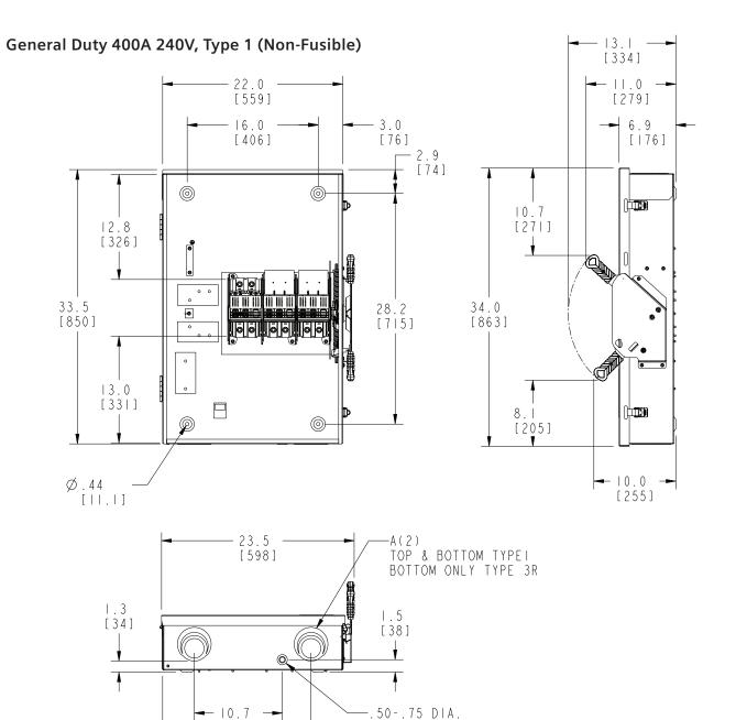
Dimensions shown in inches and millimeters [ ]. Dimensions shown accurate to  $\pm$  1/8 inch.
