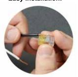
1. TURN OFF POWER. Strip wire approximately 0.45 inches. The strip length is marked on the connector.
