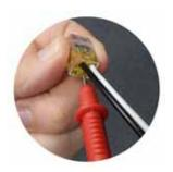
3. Use a voltage tester to test your connection via the port on the connector
