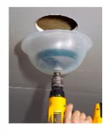
Driller's Dust Bowl solves the problem of making a mess while drilling large diameter holes in ceiling for the installation of a recessed light fixture, eliminating the need for face masks, goggles, drop cloths or vacuuming. The tool accessory easily fits between a drill's chuck and cutting tool. It forms a seal to the surface of the material being worked on and collapses like a plunger to allow the user to perform the
