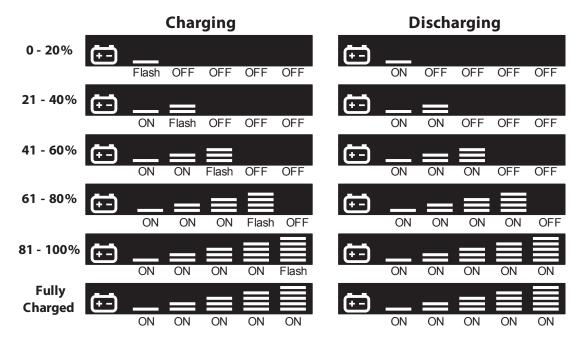
Figure 24: Battery Level indicators
