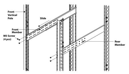
Figure 10: Installing front member of each slide rail assembly
