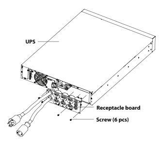
Figure 15: Removing the receptacle board
