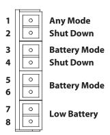
Figure 26: Terminal block layout
