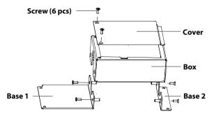
Figure 16: Splitting the box assembly
