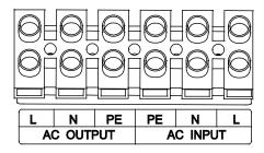
Figure 19: UPS I/O terminal block
