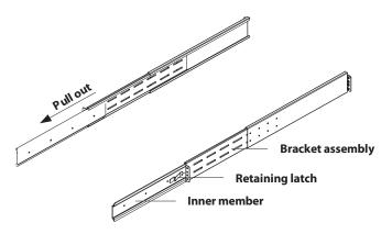
Figure 8: Pulling inner member from each bracket assembly
