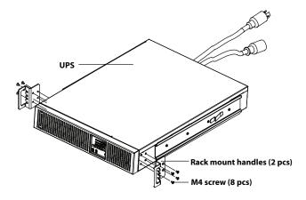
Figure 13: Installing rack mount handles
