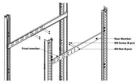
Figure 11: Fastening rear member and front member together
