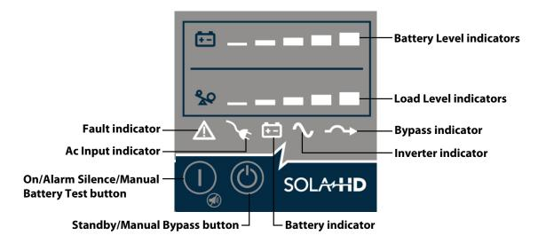
Figure 23: Operation and display panel
