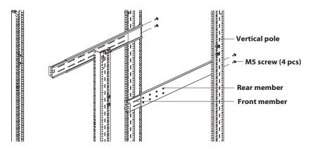
Figure 9: Installing rear member of each slide rail assembly
