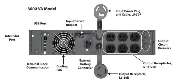
Figure 2: S4K2UC 120 V rack/tower models—rear panel components
