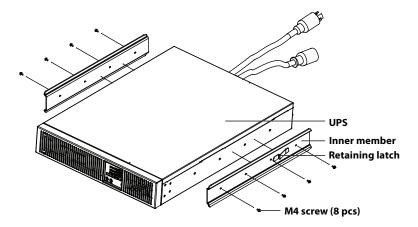
Figure 12: Installing inner members
