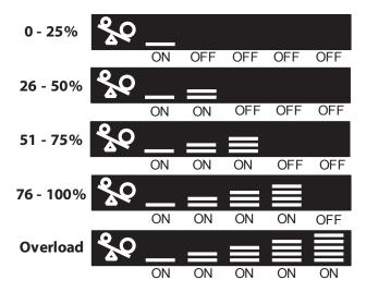
Figure 25: Load Level indicators
