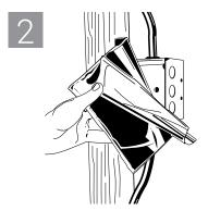
Align pad to the side of box partially overlapping the stud and adhere. Work to opposite side of the box to the edges.
