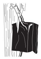
If wall membrane is in place, pack putty into gaps between box and wallboard slightly overlapping inner wallboard surface. If membrane is to be installed after pad installation, overlap front edge of box so that putty will be compressed around edges of box as wallboard is installed. Cut slits in pad to fit around conduits or cables.
