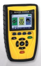
**VDV Commander™ Series** locates, tests and measures coax, data and telephone cables to ensure fast and accurate voice/data/video installations. In addition, the
