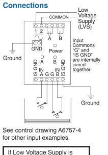
grounded, the ground must be connected to terminal 2.
