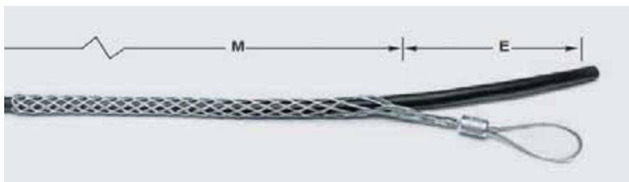
Slack Pulling Grips are offered in three styles made of galvanized steel. The closed type is used when the cable end is accessible. When not accessible, there are split lace and split rod closing styles. All grips feature a single offset eye for easy attachment to a pulling line.
